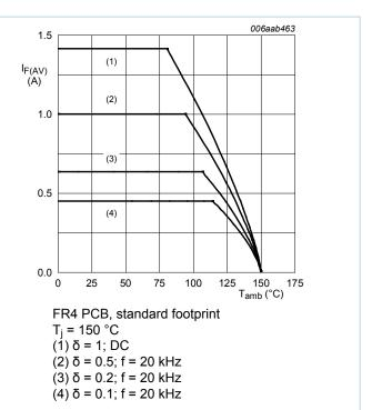
Fig. 9. Average forward current as a function of ambient temperature; typical values
