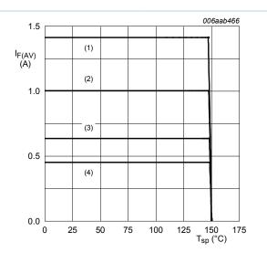
$T_j = 150 \,^{\circ}\text{C}$ (1)  $\delta = 1$ ; DC (2)  $\delta = 0.5$ ;  $f = 20 \,\text{kHz}$ (3)  $\delta = 0.2$ ;  $f = 20 \,\text{kHz}$ (4)  $\delta = 0.1$ ;  $f = 20 \,\text{kHz}$
