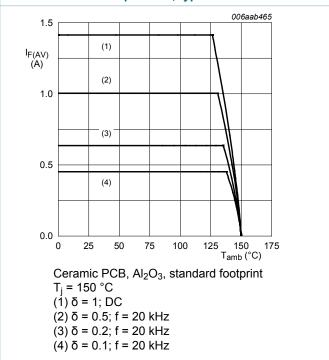
Fig. 11. Average forward current as a function of ambient temperature; typical values
