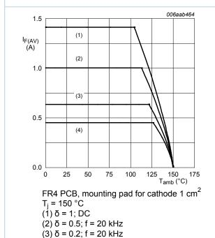
Fig. 10. Average forward current as a function of ambient temperature; typical values
